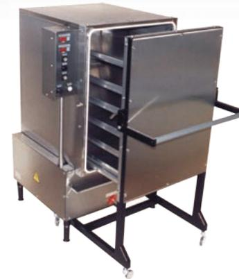
Steam cooking chamber UNIPAR U3-E is a non-pressure cooking device with electric heating, adjustable time and temperature inside the chamber and automatic water filling system. It is designed for the heat treatments of food products, especially proof dough dumplings, potato dumplings, boiling potatoes and rice, cooking meat and meat products, sterilization and defrosting meals. It is suitable for catering companies, canteens or restaurants.
