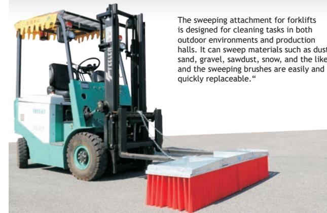
The sweeping attachment for forklifts is designed for cleaning tasks in both outdoor environments and production halls. It can sweep materials such as dust, sand, gravel, sawdust, snow, and the like, and the sweeping brushes are easily and quickly replaceable."
