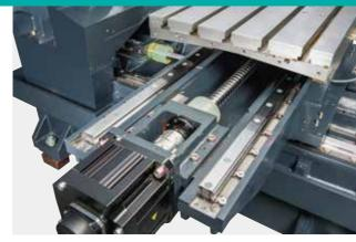
Transmission without backlash and power lost servo motor transmit power to ball screw through precision coupling.
