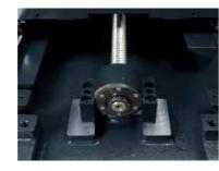
PRECISION BALLSCREWS Pretensioned ballscrews on X, Y, Z axes ensure accuracy and eliminate positioning errors.
