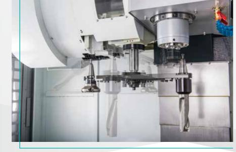
• Fast tool change ATC system T to T 1.7 Sec / 60Hz • All series are standard with 24T or 36T arm type ATC system which can easily fulfill various types of processing needs. • Rigid clamping force to make sure zero risk of tool drop.
