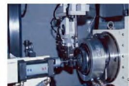
Hydraulic tailstock / The 4<sup>th</sup> axis
