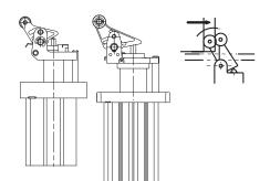
The built-in shock absorber softly catches and stops the work carrier. The strength of absorber can be easily adjusted, which makes the cylinder work in the best condition, conforming to the speed of the conveyor line and the weight of the work carrier.
