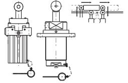
The top rollers with the built-in spring return in touch with the bottom of the work carrier. Automatically returns up to the original position as the work carrier pass by, and immediately works as a stopper for the next work carrier. Therefore the timing carriers does not need to be taken.
