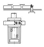
Rod and cylinder are designed for toughness against the large side load. Also suitable for the relatively slow-moving conveyor line with the heavy work carriers.
