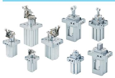
Stopper cylinders are used for safety stop or separation of objects which moves on belt, roller, chain or other conveyor. Regarding the series (see description below), the cylinders can be equipped for example with hydraulic shock absorber for soft stop of moving object, or with spring for automatic separation of two objects.
