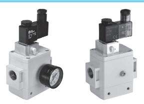
Soft start-up valve is used everywhere, where items in line behind the valve should be secured against intense pressure rise after connection to air supply, as is common when hand valve or quick connect couplings are used. When the valve is energized or manually operated, output pres-
