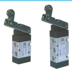
Valves are actuated by rolling the cam from the one or another side of the valve body. The cam must go over the roller and release it. During the cam return, the roller will not activate the valve. Those valves are used in pneumatic controlled circuits and everywhere where only one signal about movement is necessary. There are 3/2 normally closed and 5/2 valves available.
