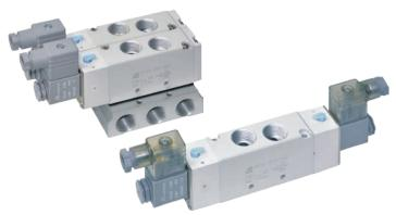
This valve series that complement favorite MVSC series with their parameters, over which they can handle up to 1.2 MPa. Other parameters, such as power consumption and flow, are the same or similar. The MVSE series is indirectly controlled. All 5/2 with one or two coils and 5/3 with medium closed, ventilated and under pressure (5/3 not available for MVSE-500) are available. The valves can be used directly or can be mounted on a manifold.
