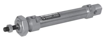
Cylinders are designed to meet the specifications of international standard ISO 6432. The cylinders can work in higher temperatures by request. Fully adjustable cushioning at end of stroke is available for diameters 20 and 25 mm, diameters 16 mm and less are without cushioning at the end of stroke. Cylinders with pressed-in tube can't be disassembled.
