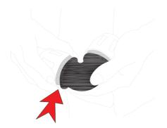
Mark the depth indicated by the socket depth meter on the pipe.
