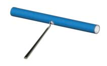
Remove the branch and clean the hole with the help of the special deburring tool
